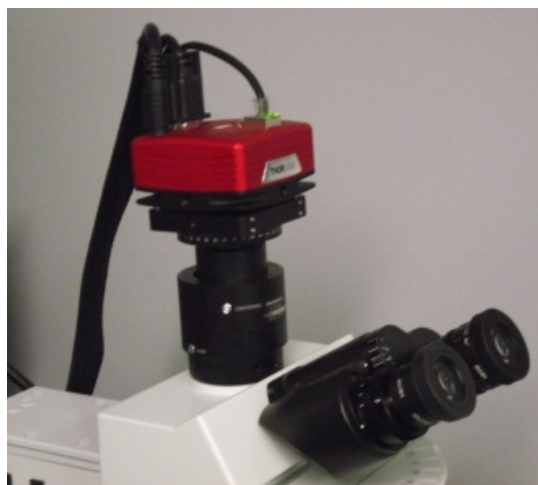
Figure 5 Camera Shown on Microscope Using C-Mount Adapter
