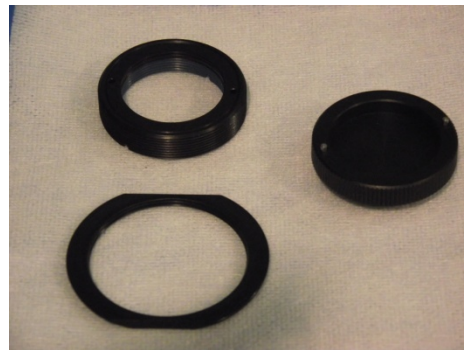
Figure 14 Removing the C-mount and IR-Block Filter Assembly from Camera Body
