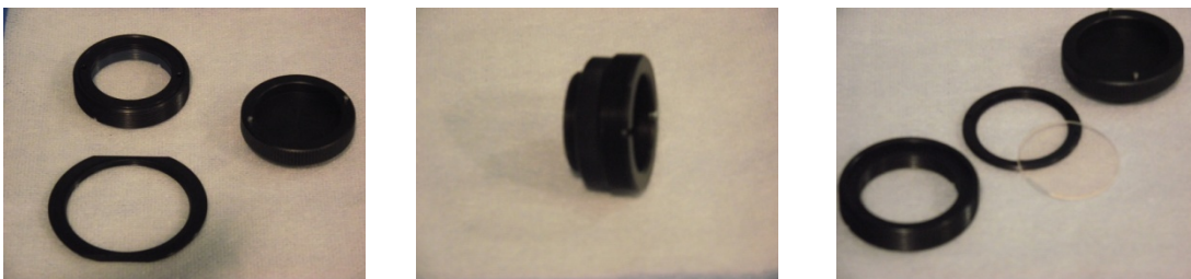
Figure 15 Removal of the IR-Blocking Filter from the Assembly
