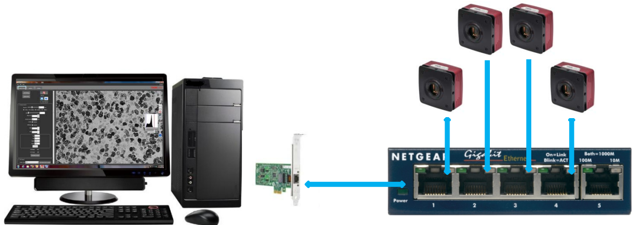
Figure 3 Gigabit Ethernet Switch Topology Setup
