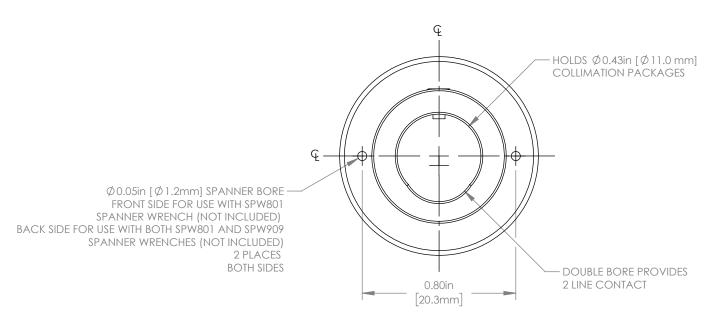
THORLARS DRAWING PROJECTION  $\bigoplus$ NAME DATE Ø11.0mm COLLIMATION TO SM1 ADAPTER CG 28/AUG/14 REDRAWN 28/OCT/14 MATERIAL APPROVAL PG REV N/A D COPYRIGHT © 2014 BY THORLABS APPROX WEIGHT ITEM # VALUES IN PARENTHESIS ARE CALCULATED 9.1 g AD11F AND MAY CONTAIN ROUNDOFF ERRORS
