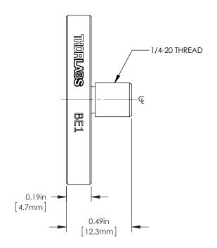
DRAWING PROJECTION  $\bigoplus$ DATE NAME PEDESTAL BASE FOR  $\emptyset$  1.00" POSTS 29/JUN/02 DAH DRAWN MATERIAL 29/JUN/02 APPROVAL AC COPYRIGHT © 2015 BY THORLABS
