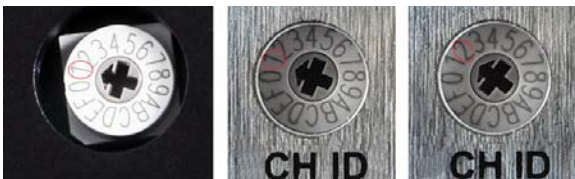
Fig. 4.1 ID switch settings
