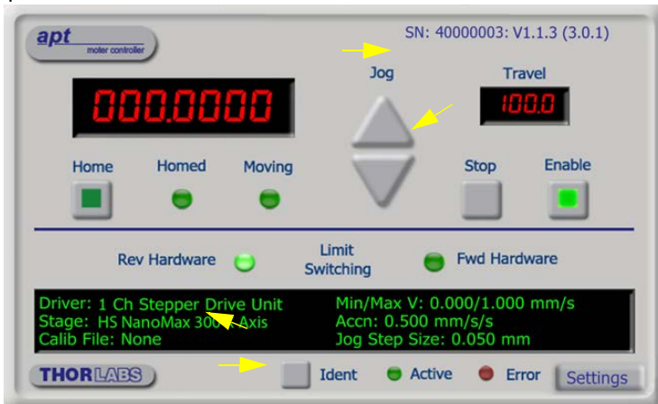
Fig. 3.4 Gui panel showing jog and ident buttons
