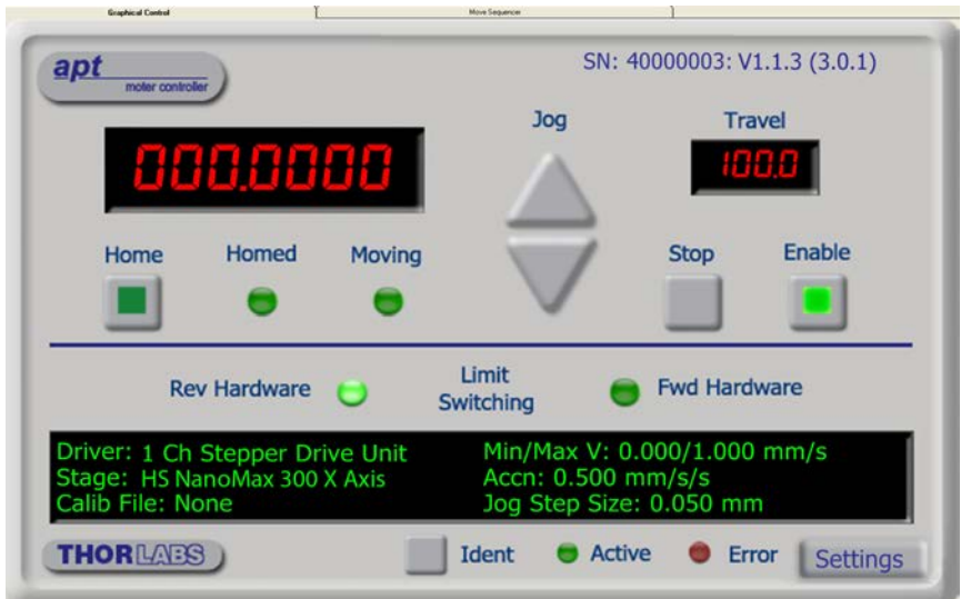
Fig. 5.1 Motor Controller Software GUI
