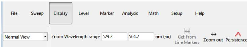
In the Display menu, the wavelength axis display can be configured.
