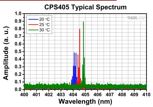
Spectrum of the CPS405 Diode Module taken at 20 °C, 25 °C, and 30 °C. The measurement was taken using Thorlabs OSA201 Spectrum Analyzer, which has a resolution of 7.5 GHz (0.25 cm<sup>-1</sup>). This data is typical and will vary for each module.
