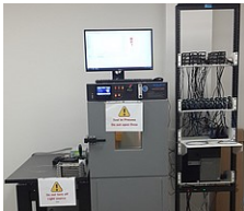
Click To Enlarge Damp Heat Testing Setup
