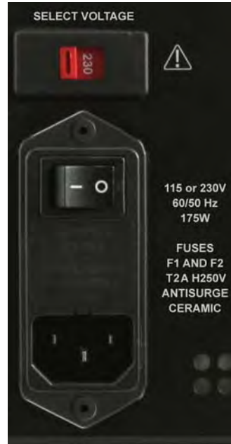
Fig. 2.3 Power Supply Unit Rear Panel
