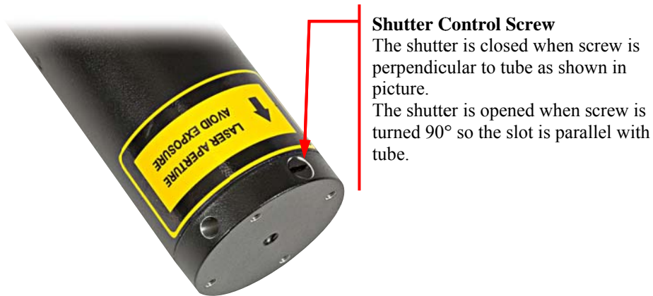
Figure 8 Laser Shutter Control, Picture shows the Shutter CLOSED.
