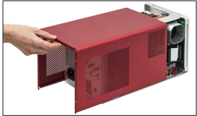
Figure 17 Slide the red cover backwards to take it out.
