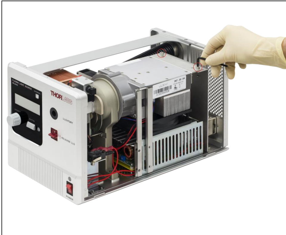
Figure 19 Remove Two Cap Screws on the Back
