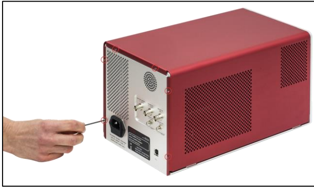
Figure 16 Remove the six screws on the back panel.
