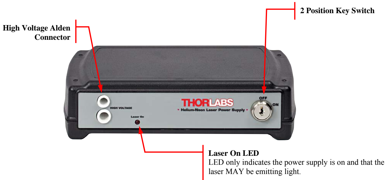
Figure 6 Front of the Power Supply Module
