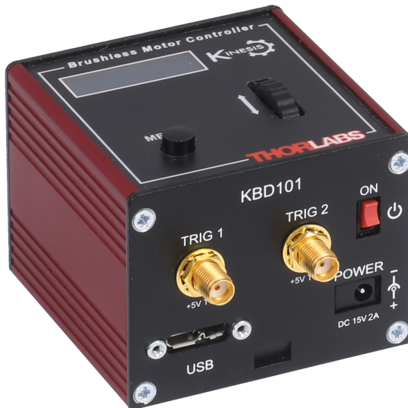
Fig. 2.1 K-Cube Brushless DC Servo Motor driver (KBD101)
