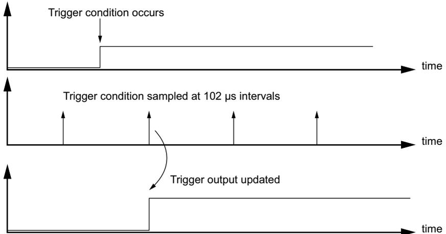
Fig. 6.11 Triggering Latency
