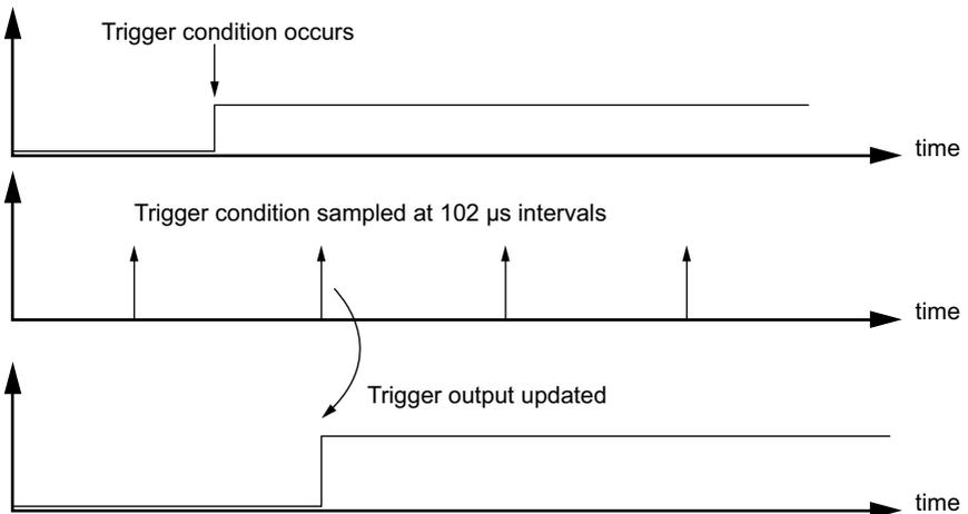
**Fig. 4.5 Triggering Latency**
