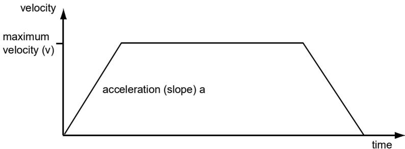
**Fig. 6.7 Graph of a trapezoidal velocity profile**
