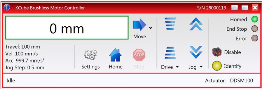
Fig. 6.1 Brushless DC Motor Driver Software GUI
