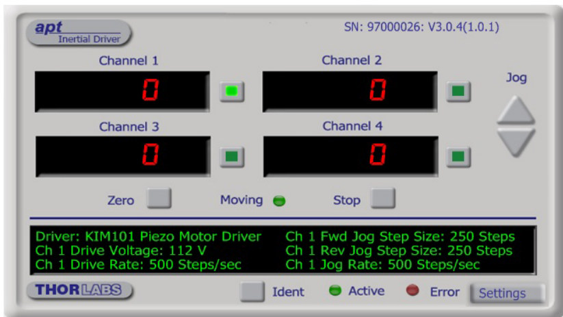
Fig. 6.1 Piezo Motor Driver K-Cube Software GUI
