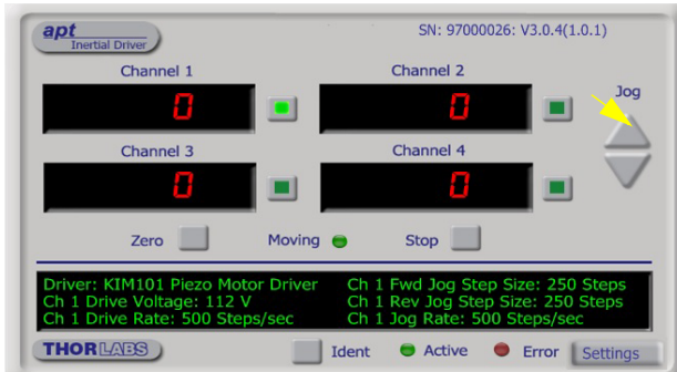
Fig. 3.5 GUI panel showing jog and ident buttons
