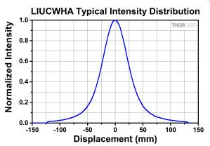
Intensity distribution of the LED in the plane located 100 mm from the LED along the emission axis.
