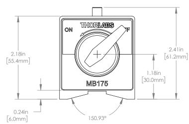
WARNING: OVER-TIGHTENING OF THE THREADED STUD WILL COMPROMISE THE FUNCTIONALITY OF THE BASE'S ON/OFF SWITCH
