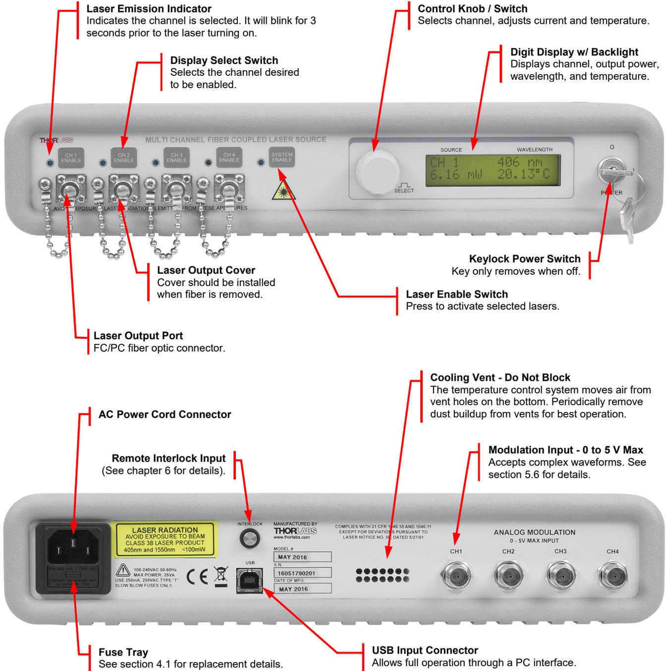
Figure 1: Front and Rear Panels of Laser Source
