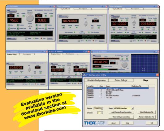
equipment manually is an important first step. Every apt<sup>TM</sup> controller can be manually operated using the supplied 'APTUser' utility. This utility gives access to all settings, parameters, and operating modes. In this way most automated alignment sequences can be first tested and verified without writing a single line of custom software by first using APTUser.
