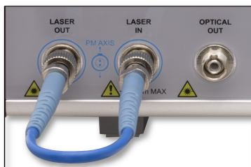
Figure 6 PM Loopback Fiber Cable Installed
