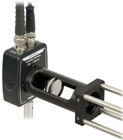
PDA series photodetector mounted onto a \varnothing 1 " Slotted Lens Tube, which is housing a focusing optic. The lens tube is attached to a 30 mm cage system via a CP02 SM1-Threaded 30 mm Cage Plate. This arrangement allows easy access for optic adjustment and signal alignment.
