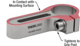
Figure 6: The POLARIS-CA1/M clamping arm has a slot that accepts a mounting screw, a separate screw that applies a clamping force to an installed post, and identical top and bottom surfaces. Since a nearly continuous track around the surface of the clamping arm is in contact with the mounting surface, clamping arms cause negligible bridging effects.
