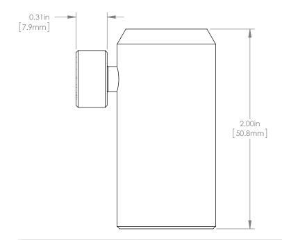
DRAWING PROJECTION THORLABS www.thorlabs.com  $(\Phi)$ NAME DATE POST HOLDER, 2" HEIGHT 23 AUG 12 ΚN REDRAWN MATERIAL REV E APPROVAL AC 24 JUN 99 N/A COPYRIGHT © 2012 BY THORLABS APPROX WEIGHT ITEM # VALUES IN PARENTHESIS ARE CALCULATED AND MAY CONTAIN ROUNDOFF ERRORS PH2 0.07 kg
