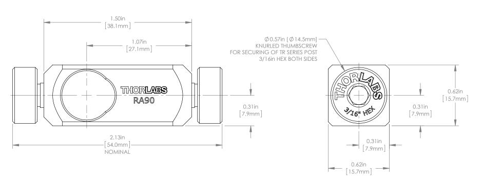
DRAWING PROJECTION  $\bigoplus$ www.thorlabs.com NAME DATE 90° POST CLAMP 15/SEP/15 REDRAWN MATERIAL rev G 27/FEB/12 APPROVAL TLB ANODIZED ALUMINUM COPYRIGHT © 2015 BY THORLABS APPROX WEIGHT ITEM # VALUES IN PARENTHESIS ARE CALCULATED AND MAY CONTAIN ROUNDOFF ERRORS 0.03 kg
