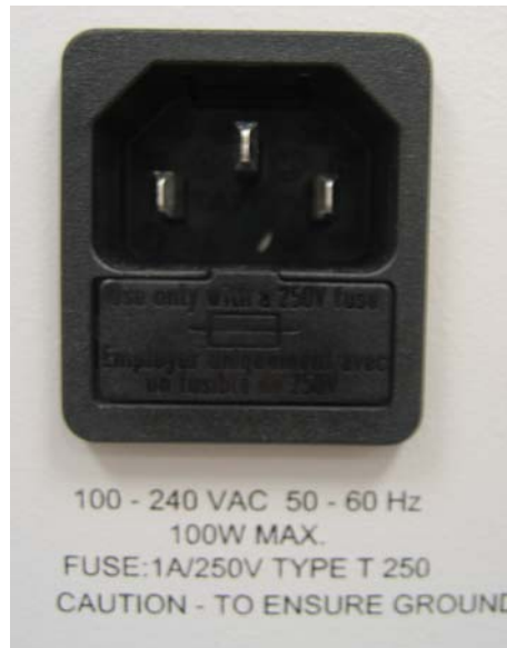
Figure 10: Fuse cover located on the Swept Source rear panel
