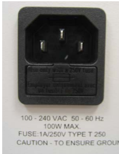
Figure 5: The AC input voltage must be 100-240 VAC and 50-60 Hz.
