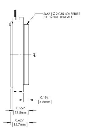
DRAWING PROJECTION  $\bigoplus$ NAME DATE **SM2 NIKON F-MOUNT** 08/JUN/15 CT REDRAWN 12/JUN/15 MATERIAL REV C APPROVAL ΗP N/A COPYRIGHT © 2015 BY THORLABS APPROX WEIGHT ITEM # VALUES IN PARENTHESIS ARE CALCULATED AND MAY CONTAIN ROUNDOFF ERRORS SM2NFM 0.05 kg
