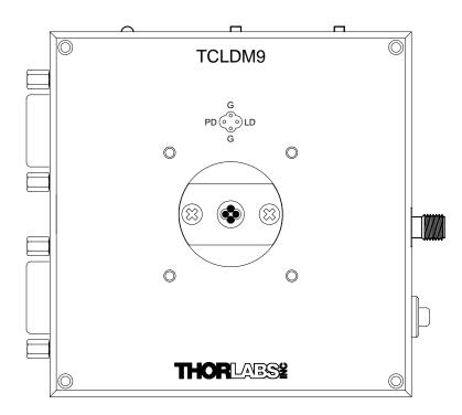
The TCLDM9 Temperature Controlled Laser Diode Mount for 5.6 and 9mm lasers allows precise temperature regulation of laser diodes. Two 13W thermo-electric coolers (TEC) provide up to 20 watts of heating or cooling power allowing the laser output power and wavelength to be easily stabilized. Both a 10K NTC thermistor and an AD592 temperature transducer are provided for temperature feedback allowing flexibility with a variety of TEC controllers.
