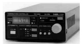
The TEC2000 thermoelectric controller has been designed for wavelength stabilization of laser diodes, and for reduced noise levels of detectors. The compact slimline chassis incorporates an adjustable PID controller with a low noise bipolar current source to drive a thermoelectric cooler element. A bi-direction output allows a single TEC element to both cool and heat. A 4 ½ - digit backlit LCD display shows the set point temperature, actual temperature, the TEC current, and the current limit.
