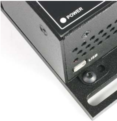
Detail A Baseplate attachment screws
