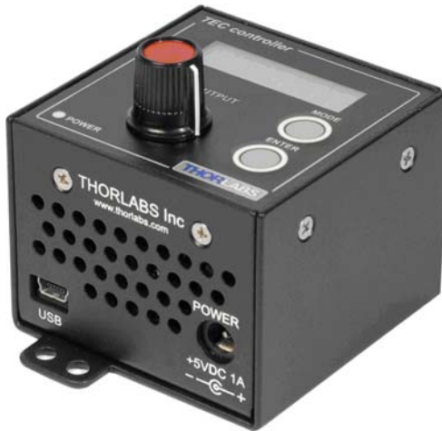
Fig. 1.1 T-Cube TEC Controller (TTC001)
