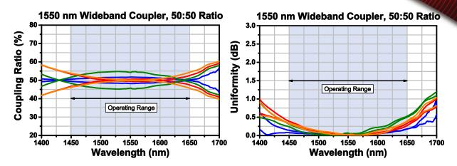
These persistence plots show the coupling ratio and uniformity performance of four TW1550R5A2 couplers (tap and signal outputs from the same coupler are indicated by matching colors on each graph). The blue-shaded region denotes the coupler's full operating wavelength range. All data was measured without connectors.
