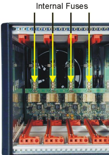
The TXP5004 must be switched off. The fuse can be replaced using tweezers or a small gripper.
