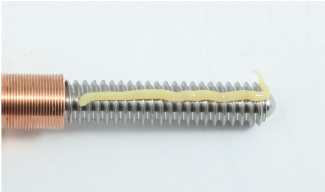
Fig. 4.1 Greasing the Leadscrew
